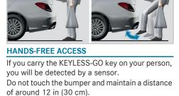
To open or close: kick into the sensor detection area below the bumper.
