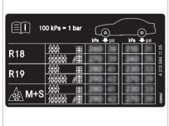
Some tire pressure tables only show the rim diameter instead of the complete tire size, e.g. **R18**. The rim diameter is part of the tire size and can be found on the tire side wall ( $\rightarrow$  page 410). Be sure to also observe the following further related subjects:
