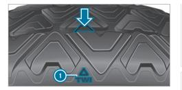
Six marks () show where the bar indicators (arrow) are integrated into the tire tread. They are visible once a tread depth of approximately 1/16 in (1.6 mm) has been reached.
