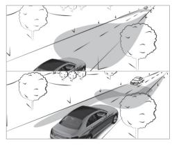
The Adaptive Highbeam Assist automatically switches between the following types of light:
