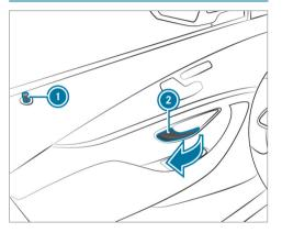
To unlock and open a front door: pull door handle (2).
