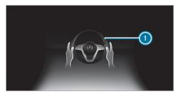
If the system detects that the driver has not steered the vehicle for a considerable period of time or has removed their hands from the steering wheel, an optical warning is given first. Display () appears in the multifunction display. If the driver still does not steer the vehicle, or gives no confirmation to the system, a warning tone sounds in addition to the visual warning message.
