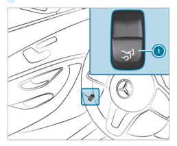
Press remote opening switch for the trunk lid
