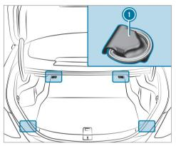
Tie-down eyes (vehicles with through-loading feature in the rear bench seat)
