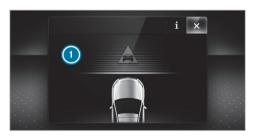
If autonomous braking or situation-dependent braking assistance has occurred, display appears in the multifunction display and then automatically goes out after a short time.
