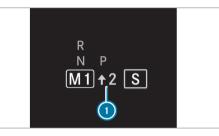
If gearshift recommendation message () is shown on the multifunction display, shift to the recommended gear.
