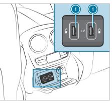
Example: USB ports in the rear passenger compartment center console
