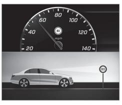
If a change in the speed limit is detected and automatic adoption of speed limits is activated, the new speed is automatically adopted as the stored speed ( $\rightarrow$  page 220).
