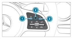
Operate the multimedia system with Touch Control (2) and associated buttons (1) and (3).
