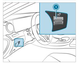
Turn brightness control ① up or down. The lighting of the Instrument Display and in the control elements of the vehicle interior is adjusted.
