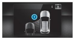
If a course-correcting brake application occurs, the red warning lamp flashes in the outside mirror and a warning tone sounds. In addition, a display () indicating the danger of a side collision appears in the multifunction display.
