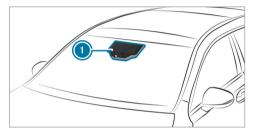
Active Lane Keeping Assist monitors the area in front of your vehicle by means of multifunction camera (). It serves to protect you against unintentionally leaving your lane. You will be warned by vibration pulses in the steering wheel and guided by a course-correcting brake application back into your lane.
