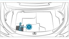
Towing eye ① is located in the stowage space under the trunk floor.
