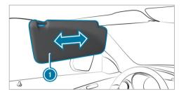
Vehicles with an extendable sun visor: slide sun visor () horizontally as required.
