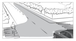
The cornering light improves the illumination of the roadway over a wide angle in the turning direction, enabling better visibility on tight bends, for example. It can be activated only when the low beam is switched on.
