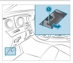
**To open:** pull lever **1** to release the hood.
