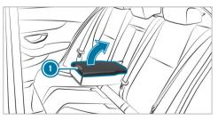
Press release catch ① and swing the cover of the armrest upwards.
