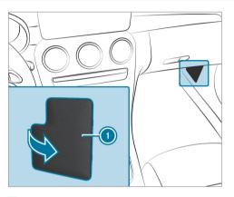
Open cover (1) in the direction of the arrow and remove it.
