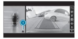
Vehicles with Blind Spot Assist: Cross Traffic Alert can warn drivers of any crossing traffic when backing up out of a parking space. The radar sensors in the bumper also monitor the area adjacent to the vehicle. If a critical situation is detected, symbol ① appears in the media display. If the driver does not respond to the warning, the vehicle's brakes can be applied automatically.
