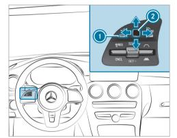
The on-board computer is operated using left-hand Touch Control 0 and left-hand back/home button 0.
