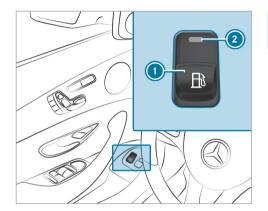
Pull button 1. Indicator lamp (2) flashes and the Please Wait Depressurizing Tank message appears in the multifunction display. The pressure in the high-pressure fuel tank is released and then the fuel filler flap opens.
