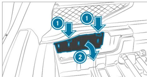
Push retaining clamps ① on the cover downwards to release them and fold out the cover in the direction of arrow ②.
