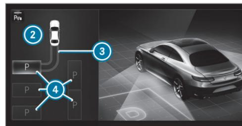
The media display shows the view of Active Parking Assist. Area ② displays detected parking spaces ④ and vehicle path ③.
