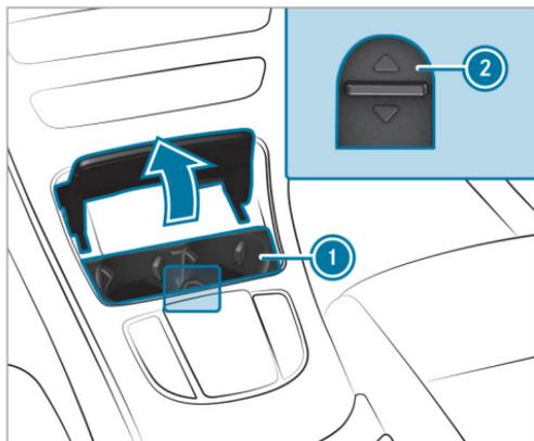
▶ **To remove:** slide catch ② forwards and pull out cup holder ①.
