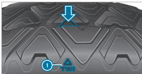
Six marks ① show where the bar indicators (arrow) are integrated into the tire tread. They are visible once a tread depth of approximately  $\frac{1}{16}$  in (1.6 mm) has been reached.
