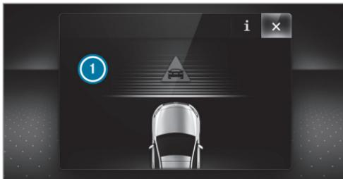
If autonomous braking or situation-dependent braking assistance has occurred, display
