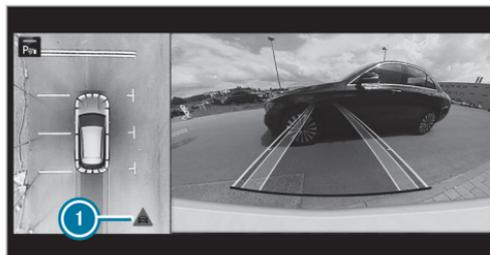
**Vehicles with Blind Spot Assist:** Cross Traffic Alert can warn drivers of any crossing traffic when backing up out of a parking space. The radar sensors in the bumper also monitor the area adjacent to the vehicle. If a critical situation is detected, symbol ❶ appears in the media display. If the driver does not respond to the warning, the vehicle's brakes can be applied automatically.
