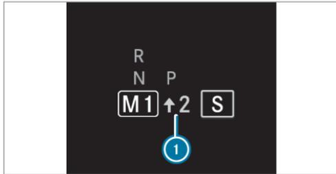
▶ If gearshift recommendation message ① is shown on the multifunction display, shift to the recommended gear.
