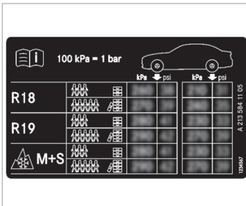
Some tire pressure tables only show the rim diameter instead of the complete tire size, e.g. **R18**. The rim diameter is part of the tire size and can be found on the tire side wall (→ page 474).
