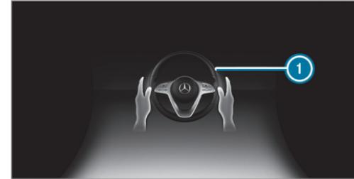
If the system detects that the driver has not steered the vehicle for a considerable period of time or has removed their hands from the steering wheel, an optical warning is given first. Display ❶ appears in the multifunction display. If the driver still does not steer the vehicle, or gives no confirmation to the system, a warning tone sounds in addition to the visual warning message.
