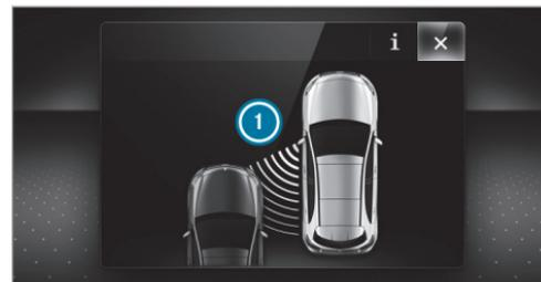
If a course-correcting brake application occurs, the red warning lamp flashes in the outside mirror and a warning tone sounds. In addition, a display **i** indicating the danger of a side collision appears in the multifunction display.
