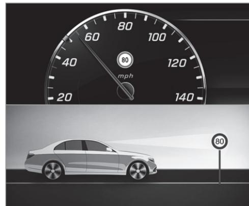
If a change in the speed limit is detected and automatic adoption of speed limits is activated, the new speed is automatically adopted as the stored speed (→ page 241).
