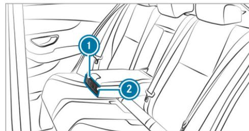
▶ **To open:** press cup holder ① or ②. Cup holder ① or ② will extend automatically.
