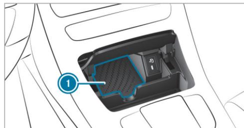
▶ Place the mobile phone as close to the center of mat ① as possible with the display facing upwards. When a message is shown in the multimedia system, the mobile phone is being charged. Malfunctions during the charging process are shown in the media display.
