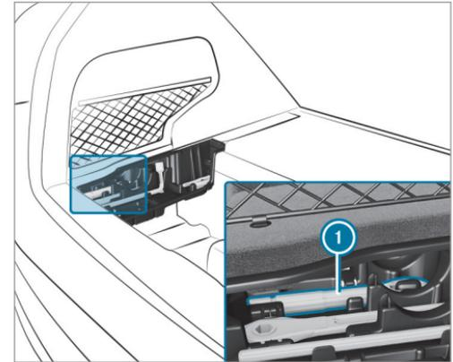
Towing eye ① is under the cargo compartment floor.
