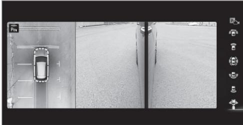
When the electrical connection is established between the vehicle and the trailer, the display changes to the side camera view.
