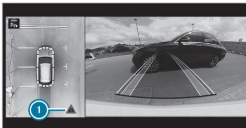
**Vehicles with Blind Spot Assist:** Cross Traffic Alert can warn drivers of any crossing traffic when backing up out of a parking space. The radar sensors in the bumper also monitor the area adjacent to the vehicle. If a critical situation is detected, symbol ① appears in the media display. If the driver does not respond to the warning, the vehicle's brakes can be applied automatically.
