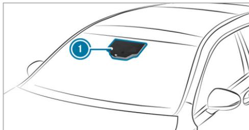
Traffic Sign Assist detects traffic signs with multifunction camera ①. It assists you by displaying detected speed limits and overtaking restrictions in the instrument cluster and optionally in the head-up display or central display.
