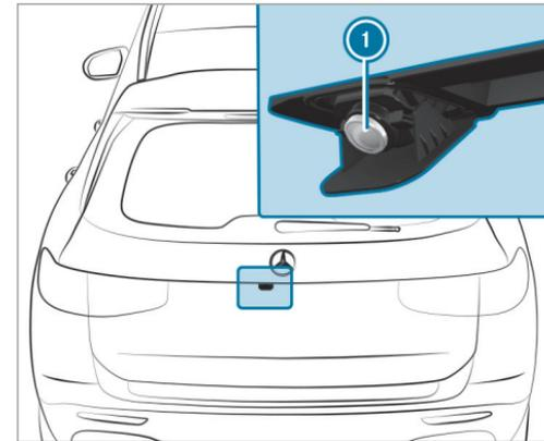
When you engage reverse gear, the image from rear view camera ① is shown in the media display. Dynamic guide lines show the path the vehicle will take with the steering wheel in its current position. This helps you to orient yourself and to avoid obstacles when backing up.
