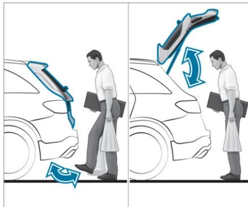
With HANDS-FREE ACCESS you can open, close or stop the closing process of the tailgate by performing a kicking movement under the rear bumper.
