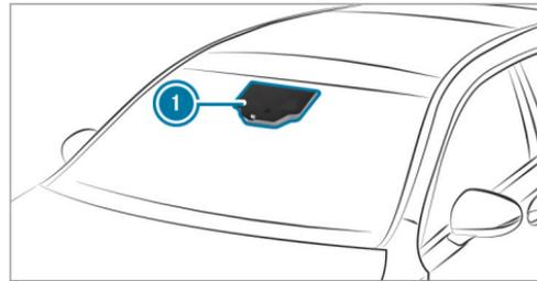
Active Lane Keeping Assist monitors the area in front of your vehicle by means of multifunction camera ①. It serves to protect you against unintentionally leaving your lane. You will be warned by vibration pulses in the steering wheel and guided by a course-correcting brake application back into your lane.
