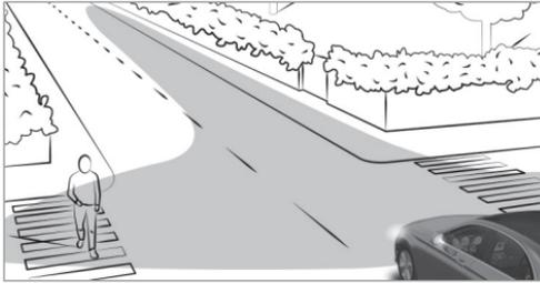
The cornering light function improves the illumination of the roadway over a wide angle in the turning direction, enabling better visibility on tight bends, for example. It can be activated only when the low beam is switched on.
