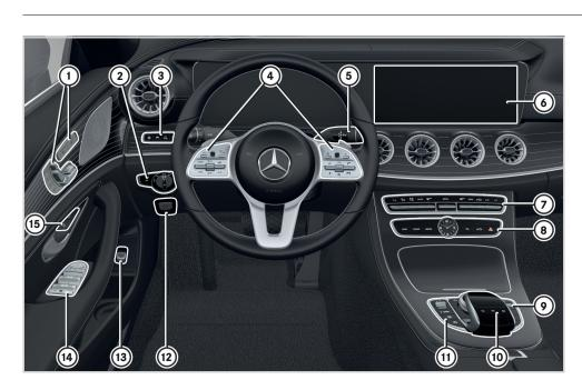
(1) Seat functions Adjusts the seat electrically Seat ventilation Adjusts the front-passenger seat Memory function and presets 1 2 3 2 Light switch 3 Driver assistance systems Active Steering Assist ✓ Active Lane Keeping Assist Switches off Parking Assist **PARKTRONIC** Depending on the equipment, the button may also be at position 11. Head-up display
