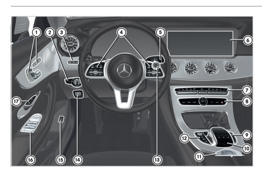
1 Seat functions Adjusts the seat electrically Seat ventilation Adjusts the front passenger seat Memory function and memory presets 1 2 3 2 Light switch 3 Driver assistance systems Active Steering Assist ✓ Active Lane Keeping Assist Switches off Parking Assist **PARKTRONIC** Depending on the vehicle's equipment, the button may also be at position 12. Head-up Display
