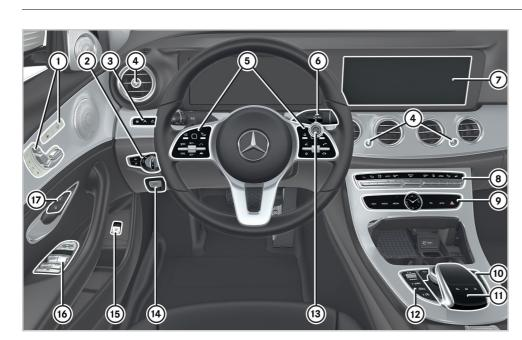
1 Seat functions Adjusts the seat electrically
