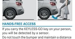
of around 12 in (30 cm). To open or close: Kick into the sensor detection area below the bumper.
