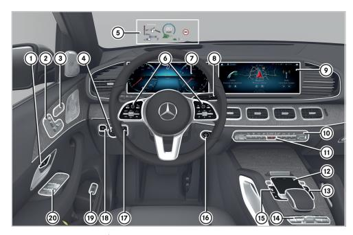
1 Door handle Locks the vehicle centrally Unlocks the vehicle centrally 2 Seat functions Adjusts the seats electrically
