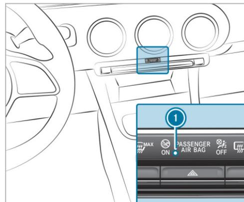
Si el sistema EDW está conectado, el testigo de control
