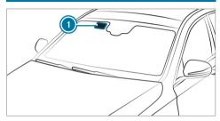
Radio-controlled equipment, e.g. toll systems, can be mounted only on areas of the windshield that are permeable to radio waves ①.
