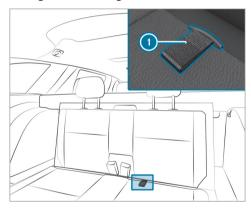
Pull the seat cushion upwards by tab and fold it back into its starting position until it engages.
