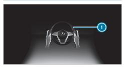
If the system detects that the driver has not steered the vehicle for a considerable period of time or has removed their hands from the steering wheel, display appears in the Instrument Display. If the driver still does not steer the vehicle, or gives no confirmation to the system, a warning tone sounds in addition to the visual warning message.
