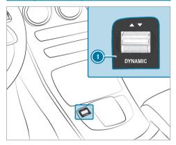
Press DYNAMIC SELECT switch forwards or backwards. The drive program selected appears in the instrument display.
