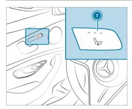
Press button repeatedly until the desired blower setting has been reached. Depending on the blower setting, up to three indicator lamps will light up. If all indicator lamps are off, the seat ventilation is switched off.
