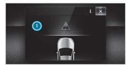
If autonomous braking or situation-dependent braking assistance has occurred, display (1) appears in the Instrument Display and then automatically goes out after a short time.
