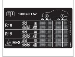
Some tire pressure tables only show the rim diameter instead of the complete tire size, e.g. **R18**. The rim diameter is part of the tire size and can be found on the tire side wall ( $\rightarrow$  page 339).
