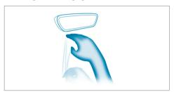
Briefly move a hand up or down beneath the inside rearview mirror. The reading light is switched on or off for the driver or the front passenger.
