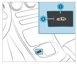
Press button 1. Indicator lamp 2 lights up. The vehicle is set to the high level. Your selection is saved.
