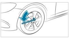
Using the lug wrench, loosen the wheel bolts on the wheel you wish to change by about one full turn. Do not unscrew the screws completely.
