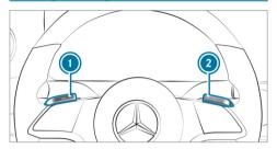
When the automatic transmission is shifted to position  $\boxed{\textbf{D}}$ , you can manually shift it with the steering wheel gearshift paddle. If permitted, the automatic transmission shifts to a higher or lower gear depending on the steering wheel gearshift paddle being pulled.
