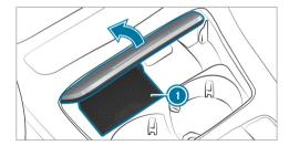
Place the mobile phone as close to the center of mat as possible with the display facing upwards.
