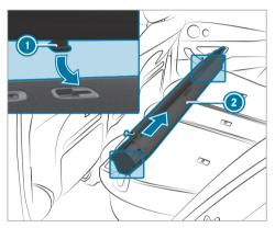
Insert combined cargo cover and net (2) into both guides 1 and push it as far as it will go in the direction of the arrow.
