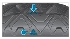
Six marks  $\bigcirc$  show where the bar indicators (arrow) are integrated into the tire tread. They are visible once a tire tread depth of approximately  $V_{16}$  in (1.6 mm) has been reached.
