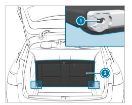
To remove: fold seat cushion 2 vertically upwards and remove it from seat cushion guide 🕦.
