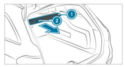
To extend: pull cargo compartment cover 1 back by handle 2 and clip it into the brackets on the left and right.
