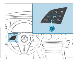
Steering wheel control panel for cruise control
