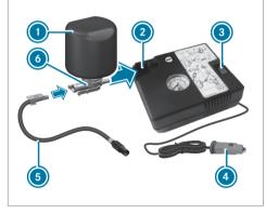
Pull plug (a) with the cable and hose (5) out of the tire inflation compressor housing.
