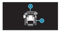
Optionally, obstacles detected by Parking Assist PARKTRONIC from a distance of approximately 3.3 ft (1.0 m) in front 2 and 2.3 ft (0.7 m) on the side (3) can also be displayed in the Head-up Display.
