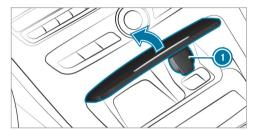
Example: 12 V socket in the storage compartment in the front center console
