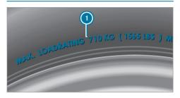
i The data shown in the image is example data. Maximum tire load is the maximum permissible weight for which the tire is approved.
