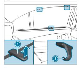
Pull the roller sunblind out by tab and hook it onto brackets at the top of the window.
