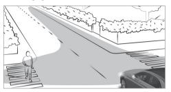
The cornering light improves the illumination of the road over a wide angle in the turning direction, enabling better visibility on tight curves, for example. It can be activated only when the low beam is switched on.
