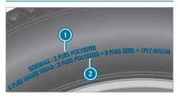
(i) The data shown in the image is example data. This information describes the type of tire cord and the number of layers in side wall 1 and under tire tread 2.
