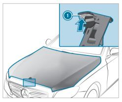
Push handle of the hood catch upwards and lift the hood until it opens automatically.
