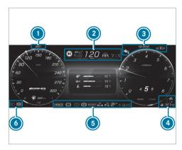
The number, positions and presentation of the status indicators on the driver's display depend on which systems are activated or deactivated.
