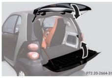
Swivel the lower tailgate upwards to close. Allow the two release levers to engage audibly. Swivel the upper tailgate downwards to close.
