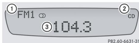
① Radio mode is activated. Depending on the waveband and the pre-set group selected, the display shows either FM 1, FM 2, AM 1 or AM 2.
