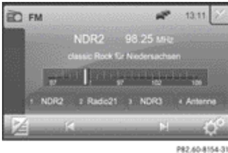
The car symbol at the top of the display indicates that announcements are switched on. If the selected station does not broadcast traffic announcements, this symbol is crossed out in red.
