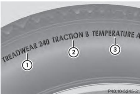
The Uniform Tire Quality Grading is a U.S. Government requirement designed to give drivers consistent and reliable information regarding tire performance. Tire manufacturers are required to grade tires based on three performance factors:
