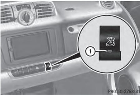
▶ **Arming:** Lock the vehicle using the remote control. Warning system indicator lamp ① flashes rapidly. The anti-theft warning system arms after about 25 seconds. When the anti-theft warning system is armed, warning system indicator lamp ① flashes about every three seconds.
