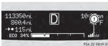
The indicator for the maximum available power of the drive system contains three segments . The number of dark segments indicates power that is currently available.
