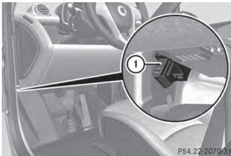
Your vehicle is equipped with a high-voltage disconnect device ① to disable the vehicle's high-voltage system.
