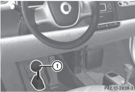
If a brake circuit has failed (▷ page 160), you must depress brake pedal ① further down to achieve the same effect and the braking distance is increased.
