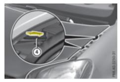
▶ Slide bars ④ on the left and right of the service cover under the bars on fender.
