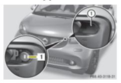
➤ To lock: insert the key into the lock and turn it to position 1.
