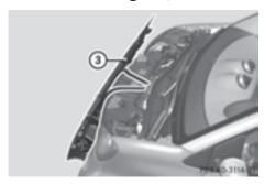
► Hook service cover ③ at the top rear in the openings on the vehicle.
