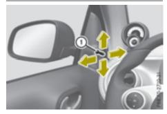
▶ To adjust the mirror: move lever (1) to the right or left, up or down.
