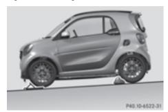
▶ On light downhill gradients: place chocks or other suitable items in front of the wheels of the front and rear axle.
