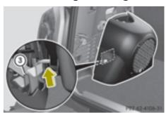
▶ Slide the subwoofer up in the direction of the arrow on bracket (3).
