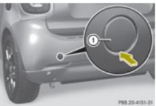
▶ Remove the towing eye from the stowage space.
