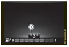
▶ Shift one gear up or down according to gearshift recommendation ① when shown
