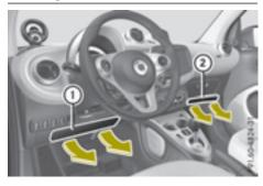
Driver's knee bag (1) deploys under the steering column and front-passenger knee bag (2) under the glove box. The driver's and frontpassenger knee bags are triggered together with the front air bags.
