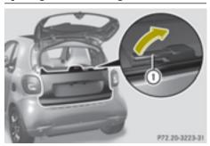
► Pull release catch ① upwards. Swing the lower tailgate down.
