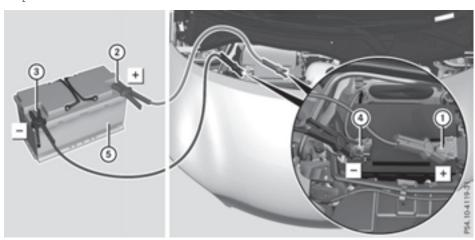
Position number 5 identifies the charged battery of the other vehicle or an equivalent jump-starting device.
