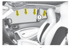
Window curtain air bags (1) are integrated into the side of the roof frame above the doors
