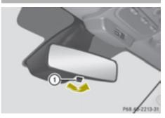
▶ Anti-glare mode: pivot anti-glare switch (1) forwards or back.
