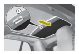
The roller sunblind shields the vehicle interior from sunlight.
