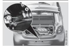
① Engine number (stamped into the crank-case)
