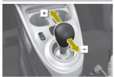
► To shift up: push the selector lever in the + direction.
