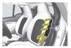
Thorax/pelvis air bags ① deploy next to the outer bolster of the seat backrest.
