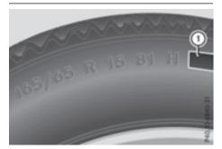
In addition to the load-bearing index, load rating ① may also be imprinted on the sidewall of the tire. This is located after the letters that identify the speed rating (> page 191).
