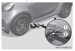
▶ Position jack ② centrally under the triangular indentations at the jacking points on the sill ①.
