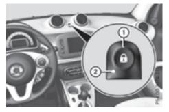
► To lock: when the vehicle is unlocked, press button  $\bigcirc$ .
