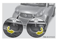
▶ Pull both levers ① with both index fingers in the direction of the arrows.
