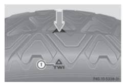
Indicator (1) shows which position the bar marking (arrow) for tread wear is integrated into the tire tread.
