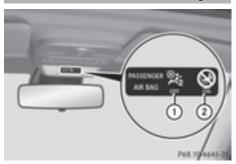
PASSENGER AIR BAG OFF indicator lamp ① and PASSENGER AIR BAG ON indicator lamp ② are part of the Occupant Classification System (OCS).
