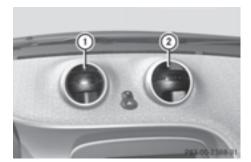
▶ To open the center air vent: hold center air vent ① or ② in the middle and tilt outwards until the vent openings can be seen.
