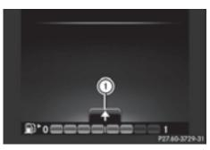
► Shift one gear up or down according to gearshift recommendation ① when shown in the multifunction display of the instrument cluster
