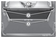
If you use the trunk cover under normal circumstances, install it in brackets (2). If you do not need to use the trunk cover, install it in brackets (3).
