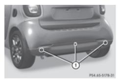
The parking aid uses three sensors ① in the rear bumper to monitor the area behind your vehicle. The sensors must be free from dirt, ice or slush. They can otherwise not function correctly. Clean the sensors regularly, taking care not to scratch or damage them.
