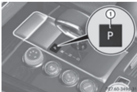
Selector lever in AMG vehicles with P button
