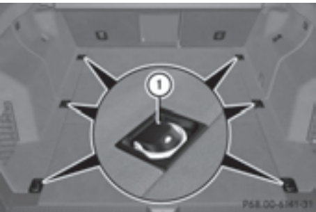
Cargo tie-down rings ① (Wagon)
