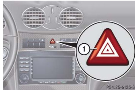
① Hazard warning flasher switch
