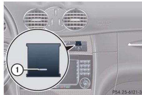
① Alarm system indicator lamp
