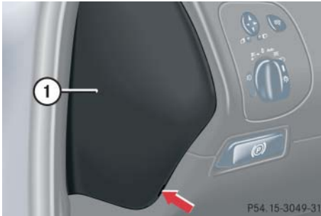
① Fuse box cover
