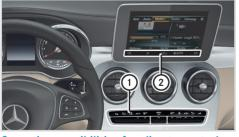
**Operating possibilities for climate control** You can set automatic climate control using: • Rocker switches on control unit (1) of the
