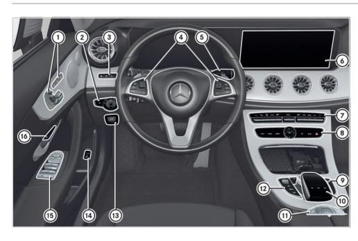
1 Seat functions Adjusts the seat electrically Seat ventilation Ls Adjusts the front-passenger seat M Memory function and presets 1 2 3
