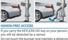
Do not touch the bumper and maintain a distance of around 12 in (30 cm). To open or close: Kick into the sensor
