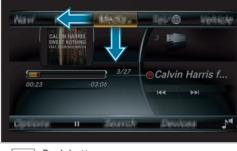
Back button Press and hold: Switches to the basic menu
