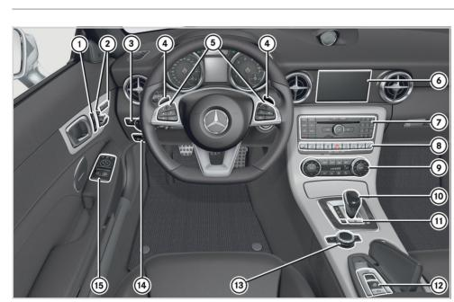
① Door handle Locks the vehicle centrally Unlocks the vehicle centrally
