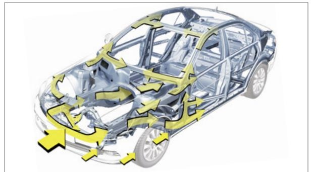
Mercedes-Benz body structures are systematically engineered to manage the forces of a variety of collision types. The basis for the high level of safety provided by a Mercedes-Benz is the fundamental principle of passive safety developed by Béla Barényi—consisting of a highly
