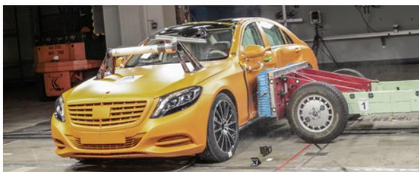
As with frontal impacts, the rigid passenger compartment is a prerequisite for effective occupant protection. In a side impact, the deformation zone available for protection of the occupants is very small in comparison to a frontal impact and requires special measures, including a very rigid side wall structure, cross-cabin reinforcements, as well as a highly effective side-impact restraint system.
