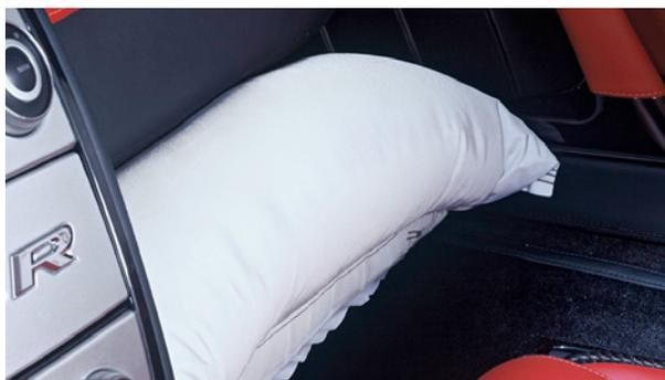
side curtain air bags are activated simultaneously on both sides of the vehicle. They are typically deployed independently of the front air bags.
