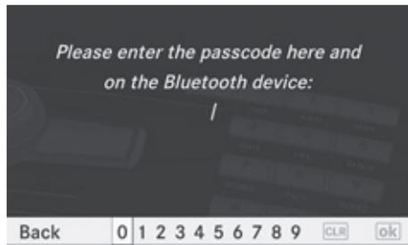
**i** The passcode is any number chosen by you between one and sixteen digits in length. We recommend to use at least four digits because this improves the quality of the encryption during connection. The passcode can differ during each authorization for each device. You must enter the same number on COMAND and on the device to be authorized. Please also refer to the instructions in the mobile phone operating guide.
