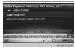
The keyword search is used to help find destinations using fragments of words. If you enable the appropriate setting in the search options, the keyword search is tolerant of errors ( $\triangleright$  page 73).
