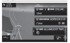
Requirement: the Highway Information map content must be enabled (> page 83). While driving on the highway, gas stations, rest stops, rest areas and highway exits are displayed along with their immediate distances from the current vehicle position.
