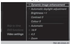
► To activate or deactivate: tick or remove the tick from the box in front of Dynamic Image Enhancement.
