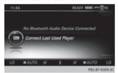
To confirm the Connect Last Used Player message in the basic display: press the controller.
