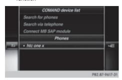
► To select a mobile phone from the device list: turn the controller and press to confirm. If the mobile phone supports the Bluetooth® PAN profile or the USB classes RNDIS, CDC/NCM or CDC/ECM, Internet access is set up. You can use the Internet functions.
