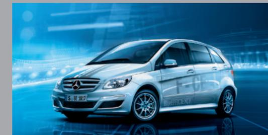
The B-Class F-CELL is locally emission-free thanks to an electric drive system which draws its energy from a fuel cell
