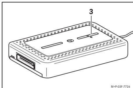
2. Press the Bluetooth® button (3) on the Media Interface Plus for approx. 3 seconds.
