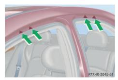
Only mount the approved roof rack to the fastening bolts (see arrows) located under the door weatherstrips.
