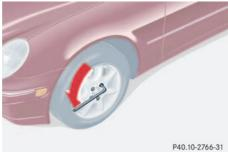
On wheel to be changed, loosen but do not yet remove the wheel bolts (approximately one full turn with wrench). The jack take-up brackets are located directly behind the front wheel housings and in front of the rear wheel housings.
