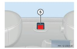
If the backrest is not locked into position, a red indicator **5** will be visible.
