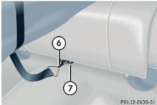
Connect snap hook 6 of front strap to eye 7 located on center tunnel in front of rear seat bench.
