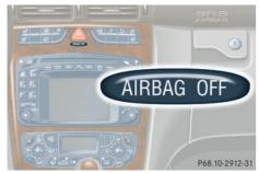
Special BabySmart<sup>TM</sup> compatible child seats, designed for use with the Mercedes-Benz system and available at any authorized Mercedes-Benz Center are required for use with the BabySmart<sup>TM</sup> airbag deactivation system. With the special child seat properly installed, the passenger front airbag will not deploy.
