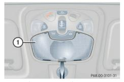
Pry of lens 1 using a flat blade screwdriver.
