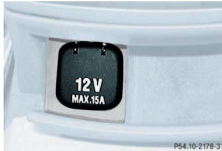
The socket is located in the rear of the center console storage compartment.
