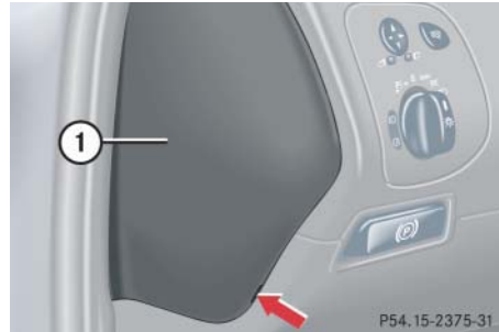
① Main fuse box cover
