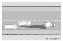
A vehicle traveling in your lane but offset from your direct line of travel may not be detected by Distronic. There will be insufficient distance to the vehicle ahead.
