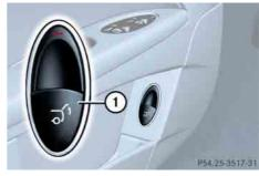
Remote tailgate release switch with indicator lamp
