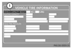
Load limit information on the Vehicle Tire Information placard The placard showing the load limit information is located on the driver's door B-pillar. If your vehicle is equipped with the Vehicle Tire Information placard (Example B), locate the heading "Vehicle Capacity Weight" on this placard. The combined weight of all occupants, cargo/luggage and trailer tongue (if applicable) should never exceed the weight listed next to vehicle capacity weight.
