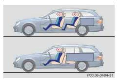
The total load weight including vehicle occupants and luggage / cargo should not exceed the load limit or vehicle capacity weight indicated on the corresponding placard which can be found on the driver's door B-pillar.
