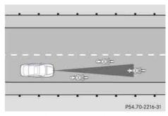
Because of its narrow profile, the vehicle traveling near the edge of the roadway has not yet been detected by Distronic. There will be insufficient distance to the vehicle ahead.
