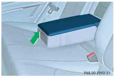
Press the handle upward and fold the armrest up.
