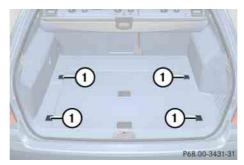
Four rings ① are located in the cargo compartment.
