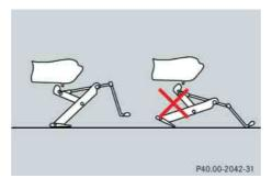
Make sure the foot of the jack is directly under the take-up bracket so that it is always vertical (plumb-line) as seen from the side, even if the vehicle is parked on an incline.
