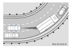
In turns or bends, Distronic may not detect a moving vehicle in front, or it may detect one too soon. This may cause your vehicle to brake late or unexpectedly.
