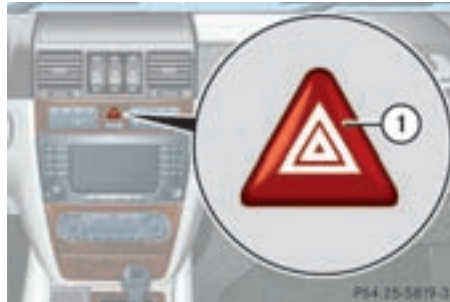
① Hazard warning flasher switch
