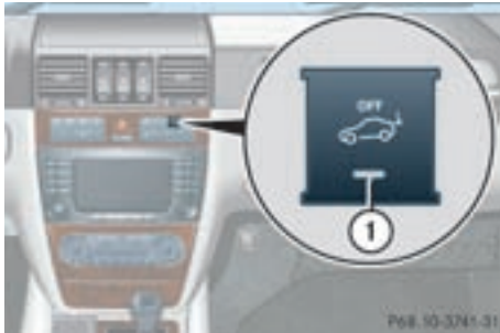
① Alarm system indicator lamp
