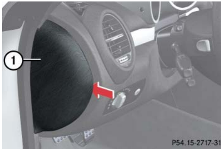
① Fuse box cover
