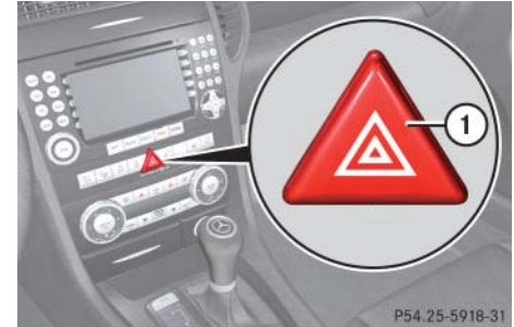
① Hazard warning flasher switch
