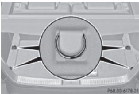
Cargo tie down rings, cargo compartment
