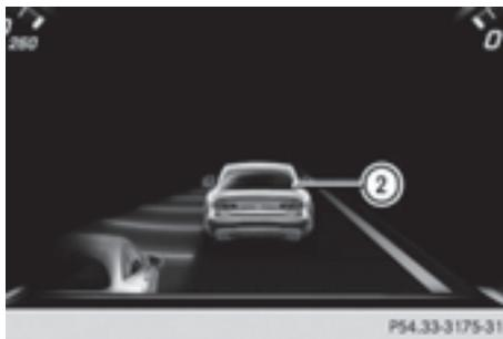
If a course-correcting brake application occurs, red warning lamp ① flashes in the exterior mirror and a dual warning tone sounds. In addition, display ② underlining the danger of a side collision appears in the multifunction display.
