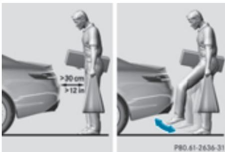
► **To open/close:** kick into sensor detection range ① under the bumper with your foot. You will hear a warning tone while the trunk lid is opening or closing.
