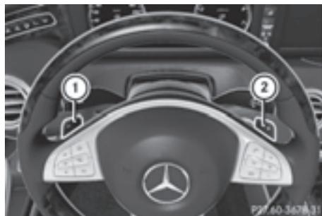
You can activate manual drive program **M** in the **E** (**C** in AMG vehicles) and **S** automatic drive programs using steering wheel paddle shifters ① and ② (▷ page 164). In manual drive program **M**, you can briefly change gear yourself by using the steering wheel paddle shifters.
