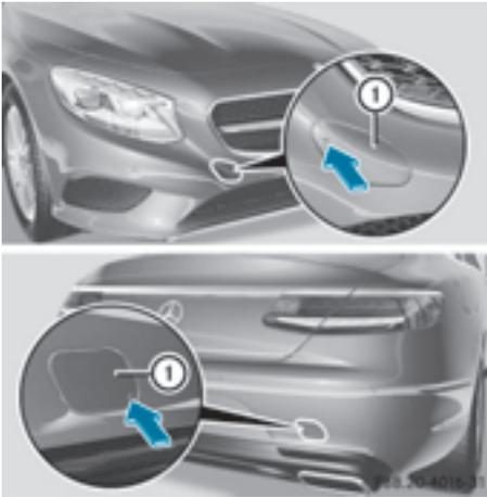
The brackets for the screw-in towing eyes are located in the bumpers. They are at the front and at the rear under covers **1**.
