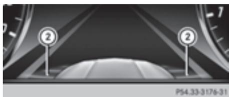
When Active Blind Spot Assist is activated, gray radar waves propagating backwards appear next to the vehicle in the assistance display. Above a speed of 20 mph (30 km/h), the color of the radar waves in the assistance display changes to green ②. Active Blind Spot Assist is then ready for use.
