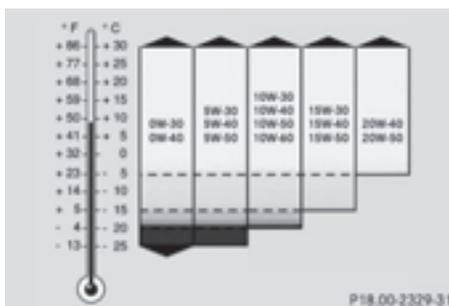
Viscosity describes the flow characteristics of a fluid. If an engine oil has a high viscosity, this means that it is thick; a low viscosity means that it is thin.
