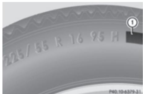
In addition to the load-bearing index, load index ① may also be imprinted on the sidewall of the tire. You will find this after the let-
