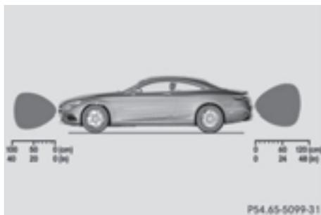
The sensors must be free from dirt, ice or slush. They can otherwise not function correctly. Clean the sensors regularly, taking care not to scratch or damage them (> page 335).
