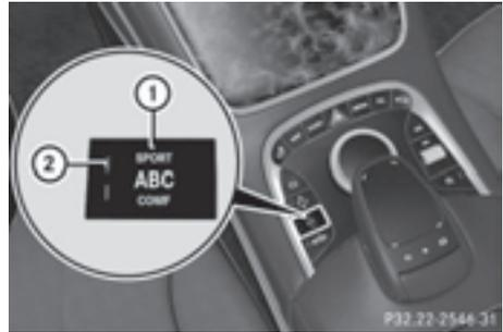
The firmer suspension setting in SPORT mode ensures even better contact with the road. The steering response behavior is sporty. Select this mode on winding country roads or highways, for example.
