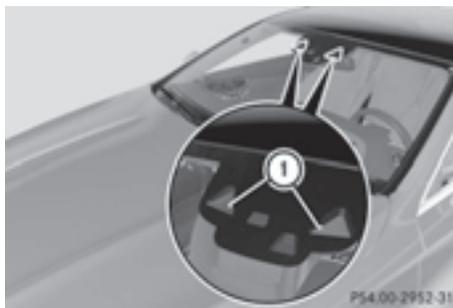
The ROAD SURFACE SCAN function monitors the road in front of the vehicle using multifunction camera ① at the top of the windshield. This function is automatically active if you select comfort suspension tuning. The system is operational at speeds of up to 81 mph (130 km/h).
