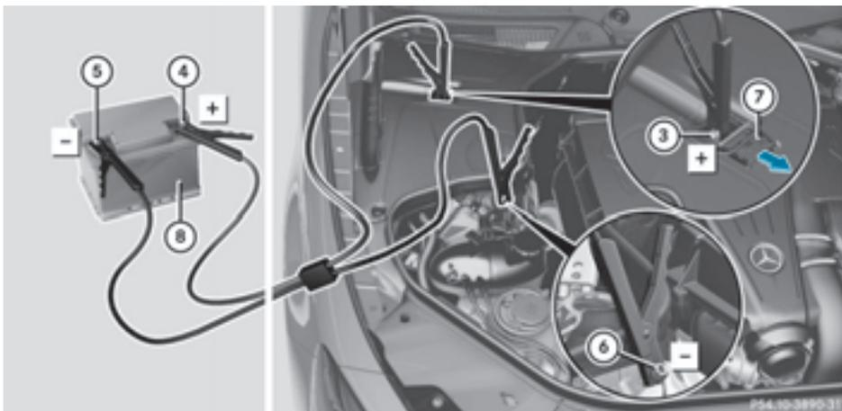
Position number ⑧ identifies the charged battery of the other vehicle or an equivalent jump-starting device.
