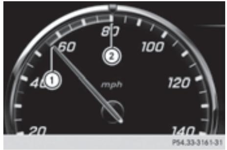
When you switch on DISTRONIC PLUS, triangle ② shows the stored speed.
