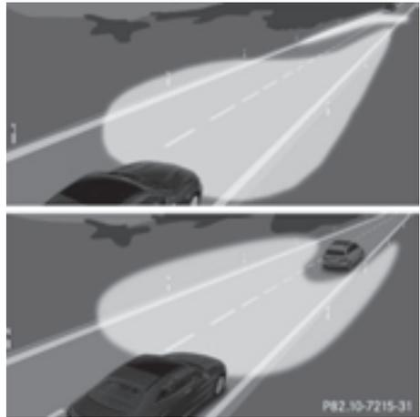
With Adaptive Highbeam Assist Plus, you can automatically switch between low-beam, partial high-beam and high-beam headlamps.
