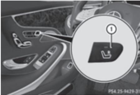
The SmartKey must be in the ignition lock and in position 1 or 2, in order for the front-passenger seat to be selected (> page 151).
