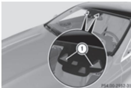
DISTRONIC PLUS with Steering Assist and Stop&Go Pilot aids you in keeping the vehicle in the center of the driving lane by means of moderate steering interventions at speeds of 0 - 125 mph (0 - 200 km/h).
