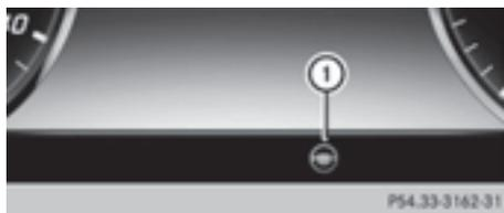
If Steering Assist and Stop&Go Pilot are activated but not ready for a steering intervention, steering wheel symbol (1) appears in gray. If the system provides you with support by means of steering interventions, symbol (1) is shown in green.
