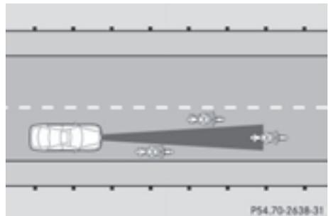
DISTRONIC PLUS has not yet detected the vehicle in front on the edge of the road, because of its narrow width. The distance to the vehicle in front will be too short.
