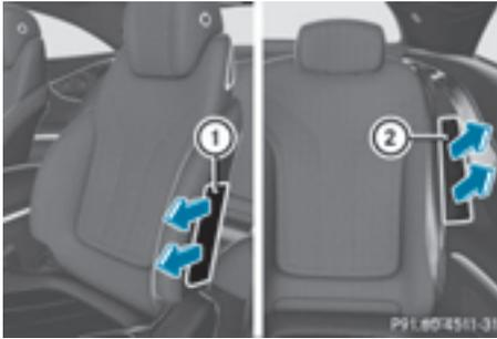
Front side impact air bags ① and rear side impact air bags ② deploy next to the outer bolster of the seat backrest.
