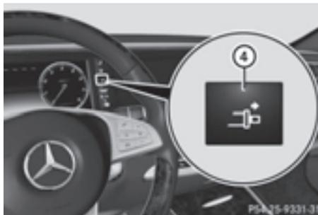
You can also extend seat-belt extender ③ with seat-belt extender button ④.
