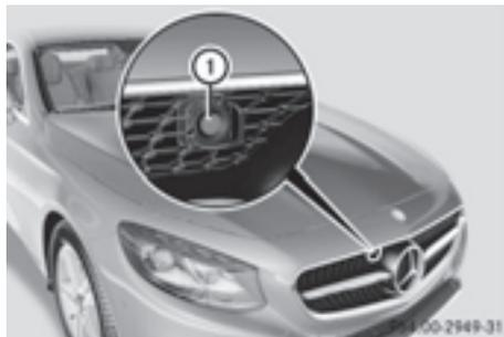
Camera lens ① is cleaned at regular intervals by operating the windshield washer system.
