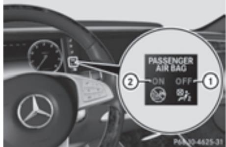
PASSENGER AIR BAG OFF indicator lamp ① and PASSENGER AIR BAG ON indicator lamp ② are part of the Occupant Classification System (OCS).
