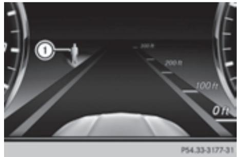
Pedestrian symbol ① in the assistance graphic indicates the status of the spotlight function. If the symbol is displayed not filled in, the function is switched on. If the symbol is displayed filled in, the conditions for the spotlight function are met.
