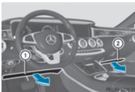
Driver's knee bag ① deploys under the steering column and front-passenger knee bag ② under the glove box. The driver's and front-passenger knee bags are triggered together with the front air bags.
