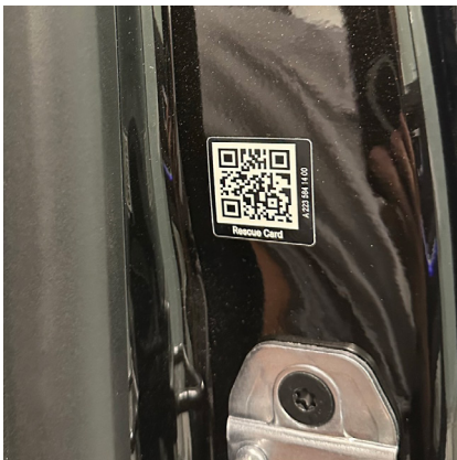
Rescue QR Code Location B-Pillar, on the opposite side of the fuel/EV socket flap
